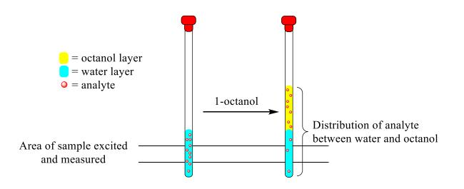
Figure 1. Representative diagram of analyte distribution between the water and 1-octanol layers upon addition of 1-octanol.
