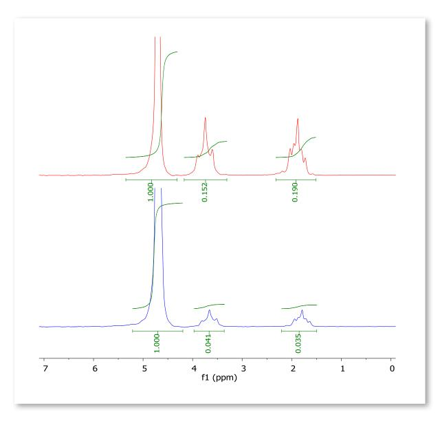
Figure 4. Spectrum of THF in water (top) and with a layer of 1-octanol (bottom).
