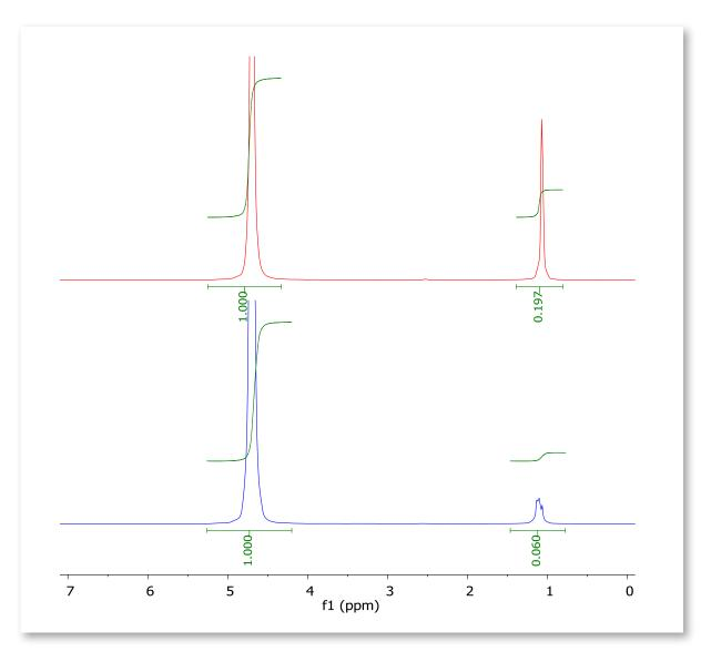
Figure 5. Spectrum of *tert*-butanol in water (top) and with a layer of 1-octanol (bottom).
