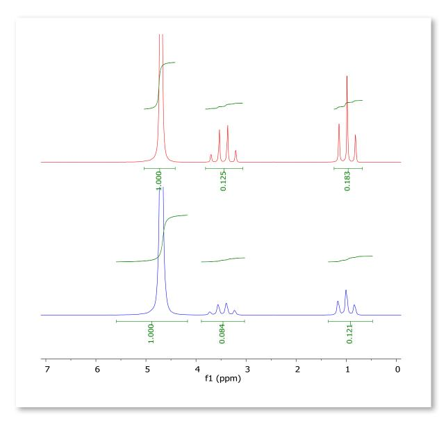
Figure 3. Spectrum of ethanol in water (top) and with a layer of 1-octanol (bottom).
