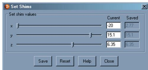
Figure 4.4 The set shims dialog with the x axis shim set to a non-ideal value
