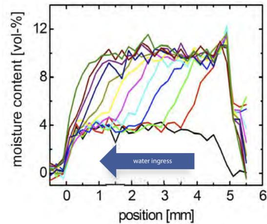
The figure at the bottom shows moisture profiles measured through a 5 mm thick concrete sample during a drying process. It can be observed how the amplitude of the uniform profile measured for the saturated sample decreases from the edges to the center until it equilibrates with the room humidity.
