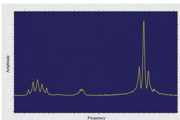
Heteronuclear  $J$ -couplings observed simultaneously between  $^{19}\text{F}$  and  $^1\text{H}$  in 1,4-difluorobenzene. The four-proton triplet is observed on the right at 2425 Hz and two atom  $^{19}\text{F}$  quintuplet at 2275 Hz on the left. (A 50 Hz noise harmonic is visible near the centre.)
