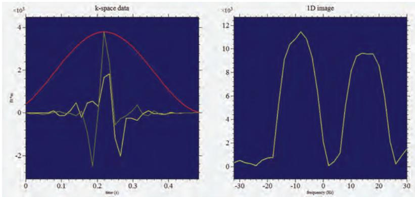
A 1D imaging sequence using a spin echo and a single gradient. On the left is the acquired echo and on the right is the Fourier transform of the echo showing the 1D projection image. The sample shown here is the two tube phantom supplied with the Terranova-MRI.
