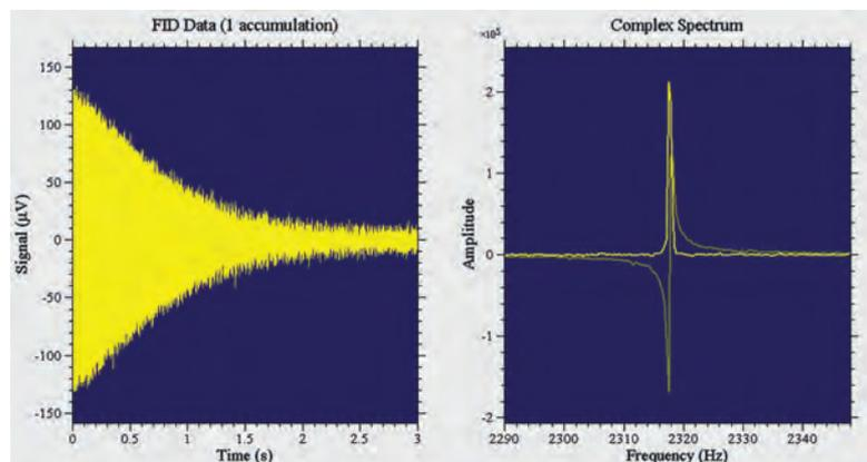
An FID of a water sample collected for 3 seconds to show the enhanced amplitude and linewidth obtained following shimming and tuning. (Note that the data has been processed in complex rather than magnitude mode - this enables the linewidth to be correctly determined).
