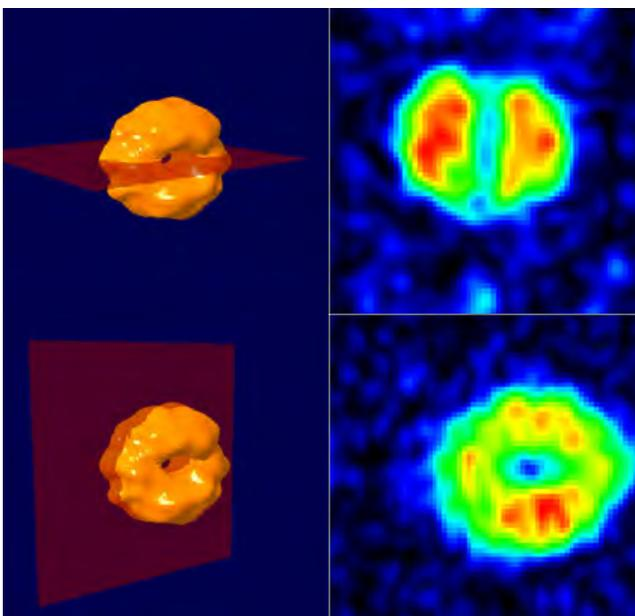
Surface renderings of a gradient-echo image of a mandarin (32 x 32 x 32 pixels) with 2D cross-sections shown to the right. Total imaging time was 4 hours with an isotropic field of view of 110 mm.
